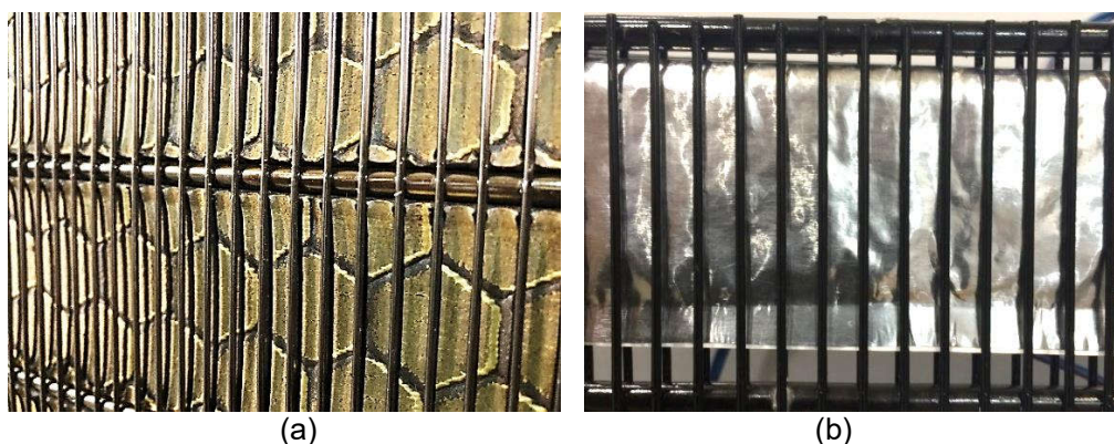
Figure 5: Condenser attachment with (a) bitumen and (b) water bags
